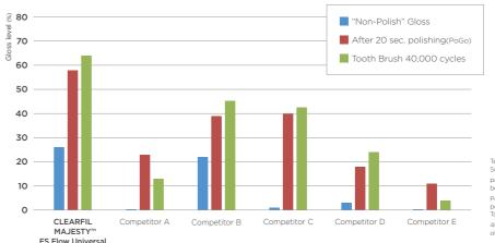
Test conditions: Specimen ø10 mm, thickness 2 mm. Surface roughened with #600 water-resistant abrasive
